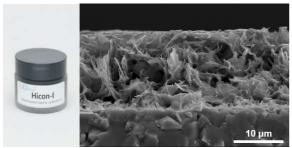
Volatile/Flexible/Conductive Graphene Ink
