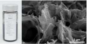
Volatile/Flexible/Conductive Graphene Liquid for Spray
